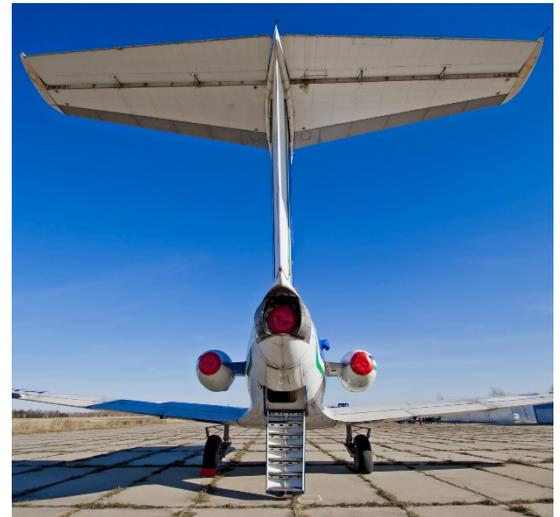
Rear view of the aircraft, showing the rear integrated airstairs
