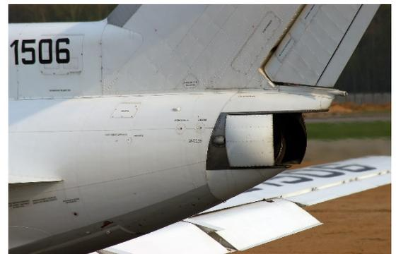
Bucket thrust reverser on the center engine
